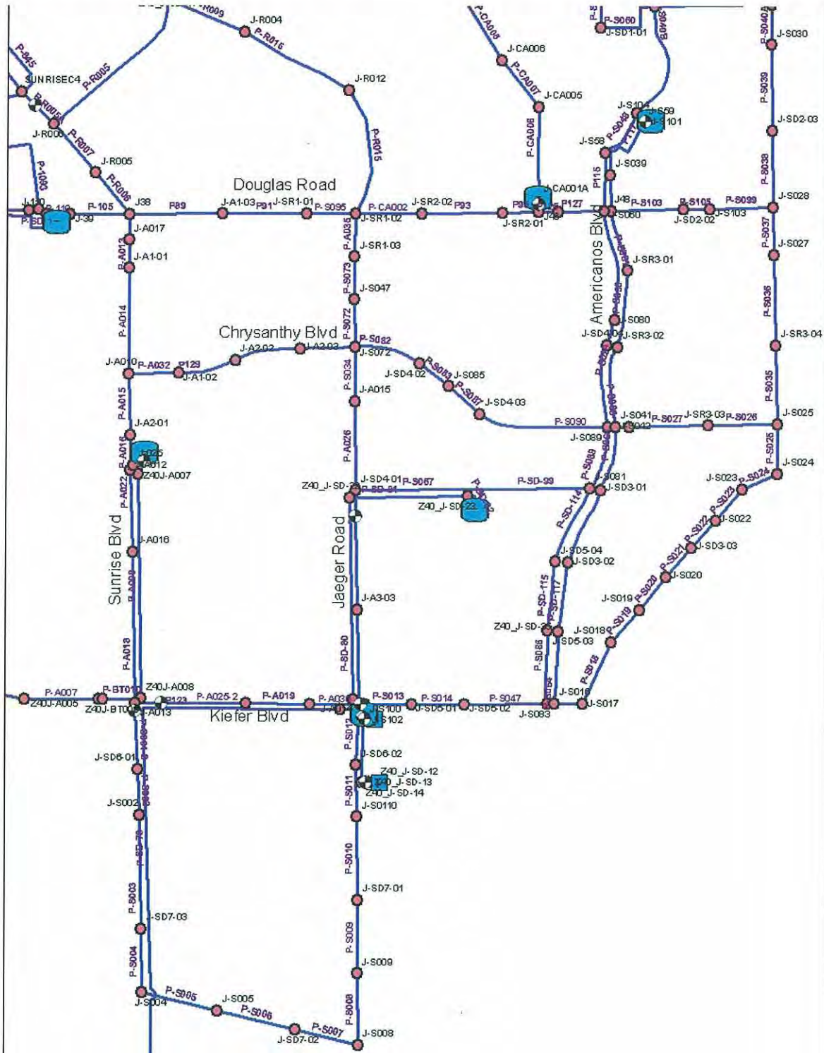
Figure A-2. Nodes and Pipes IDs in the Water Supply Phase 2 Model
