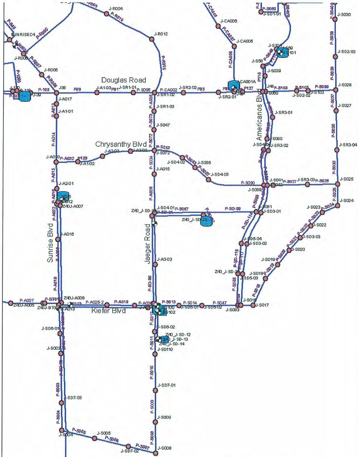
Figure A-3. Nodes and Pipes IDs in the Water Supply Phase 3 Model
