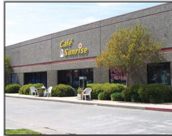
Don't Do This: This café located in Rancho Cordova does not have an adequate public space for outdoor seating. There is no shade structure or dedicated area outside of the pedestrian right-of-way designated for seating.
