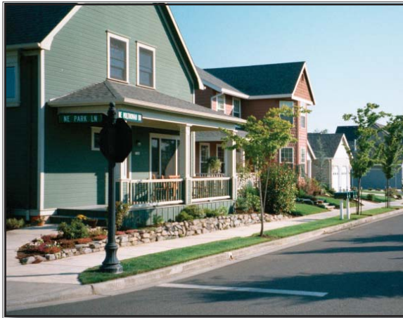
Do This: This single family project has variation in scale and massing by utilizing varying roofplanes and staggered front setbacks (Portland, Oregon).
