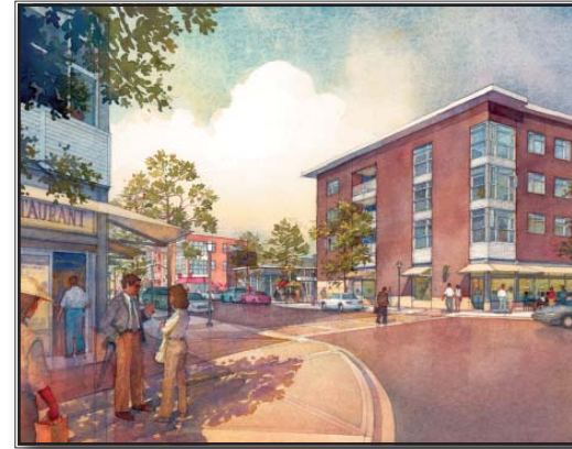
Conceptual illustration of a streetscape where buildings are close to the street, there are wide sidewalks, on-street parking is provided, street trees soften the look and feel of the street, and there are a multitude of opportunities for pedestrian interaction. Street crossings are called out with special pavement. (Courtesy LPA)
