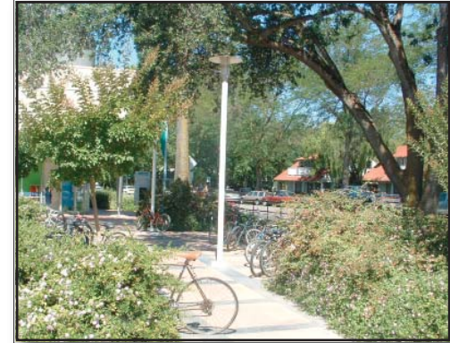
Bike parking area in Davis, California. The bike racks are located close to the street and next to the stores and offices for easy access. There is plenty of separation between the racks so that riders can maneuver their bikes around the parking area. Lighting is included for night access.
