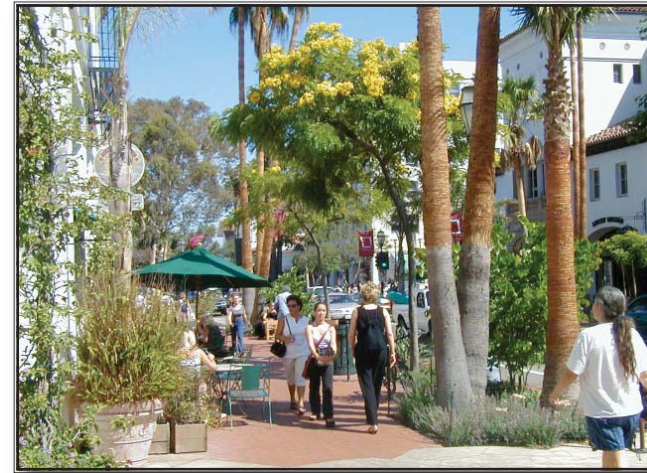
The pedestrian sidewalk of State Street in Santa Barbara, California. The street is an interesting and dynamic place to walk, with wide sidewalks, changes in paving texture and color, landscaping, street furniture (benches, trash cans, light fixtures, tables and chairs), and buildings that come right up to the back of the sidewalk.
