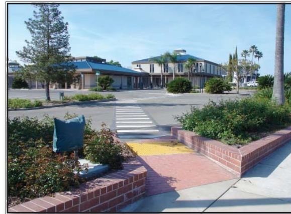
Don't Do This: Although clearly delineated this pathway winds through a large parking lot with no physical protection provided to pedestrians from vehicular traffic such as a raised walkway, landscaping, special paving or other techniques (Citrus Heights, California).
