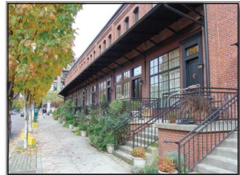
Town homes are adjacent to and accessible from the public sidewalk in this example from Portland, Oregon. The individual entries are elevated from the street to provide privacy and a transition between public and private space.
