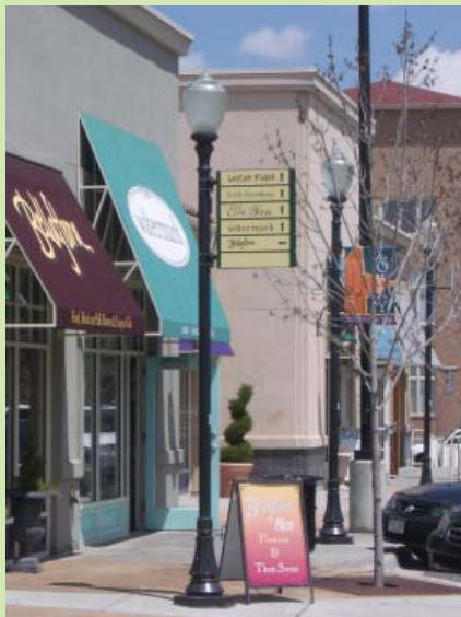
Lighting and signage may be combined into one element to reduce clutter.
