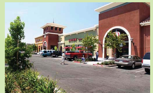
Roof and building articulation reduces building mass
