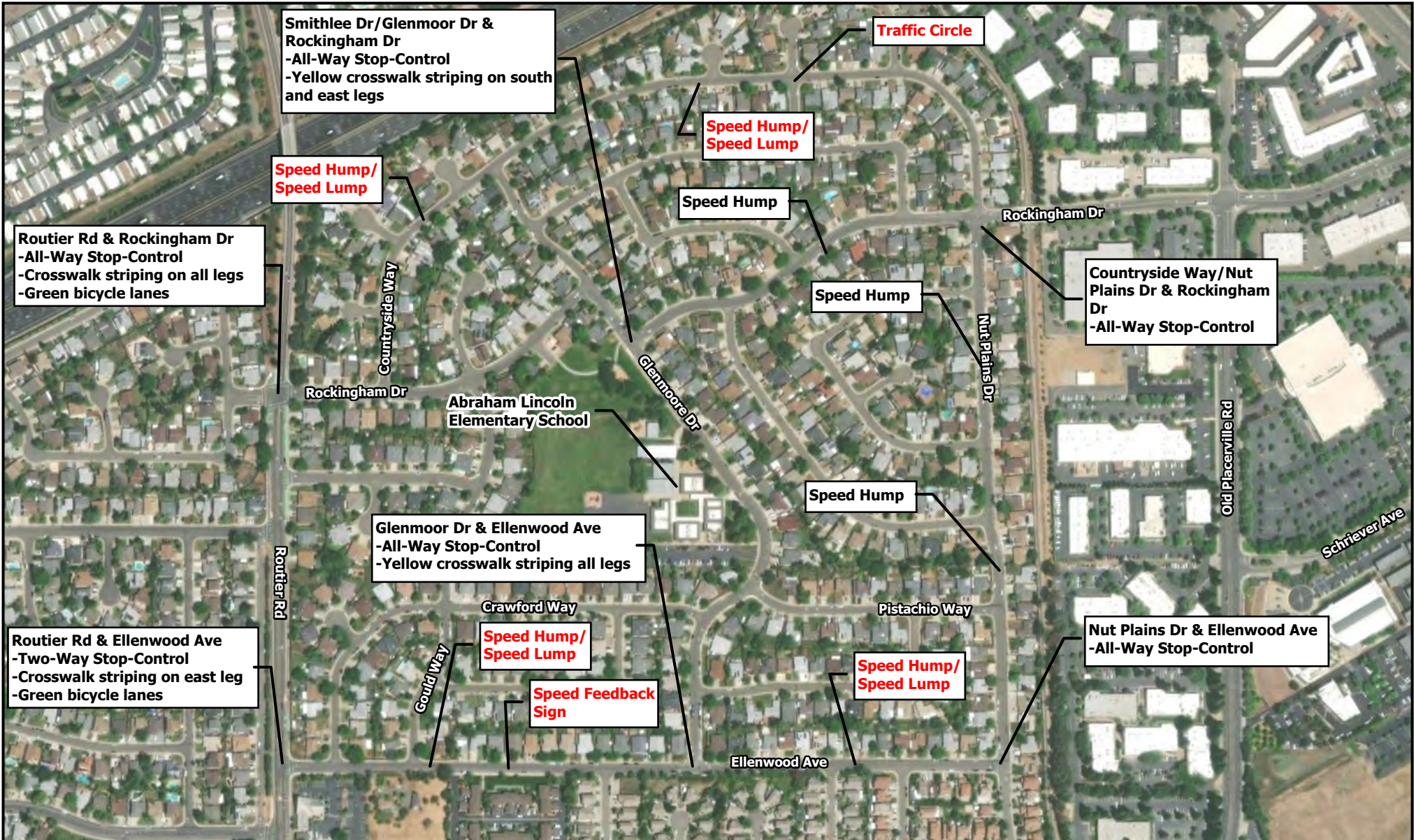
FIGURE 7 EXISTING TRAFFIC CALMING MEASURES ABRAHAM LINCOLN ELEMENTARY SCHOOL NEIGHBORHOOD RANCHO CORDOVA TRAFFIC CALMING STUDY AND CUT-THROUGH TRAFFIC ANALYSIS RANCHO CORDOVA, CA AUGUST 2024
