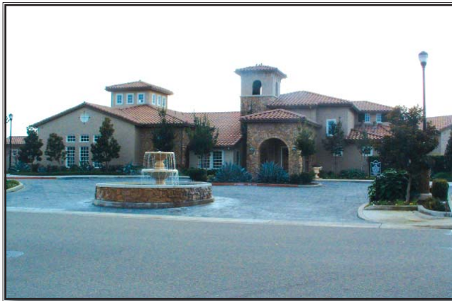
Do This: Special paving identifies shared pedestrian vehicle area for this community center building (Sacramento, California).
