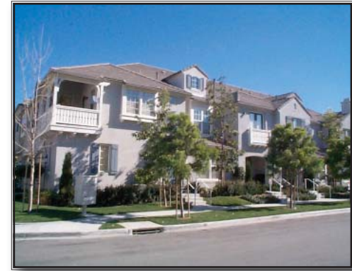
Dormers and balconies can be used to break up the perceived mass of buildings.
