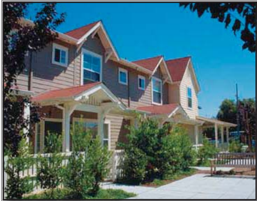
Example of a small multi-family project. Each entrance is accentuated and the roofline is broken up to reduce the potential for monotony.
