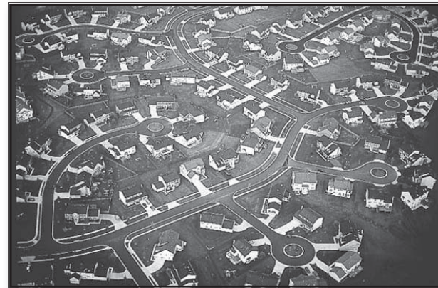
Don't Do This: Conventional cul-de-sac development with a curvilinear street system that disconnects individual residents and prohibits easy navigation of the subdivision.
